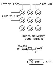
PRE-FABRICATED RAISED TRUNCATED DOME DETECTABLE WARNING SURFACE
